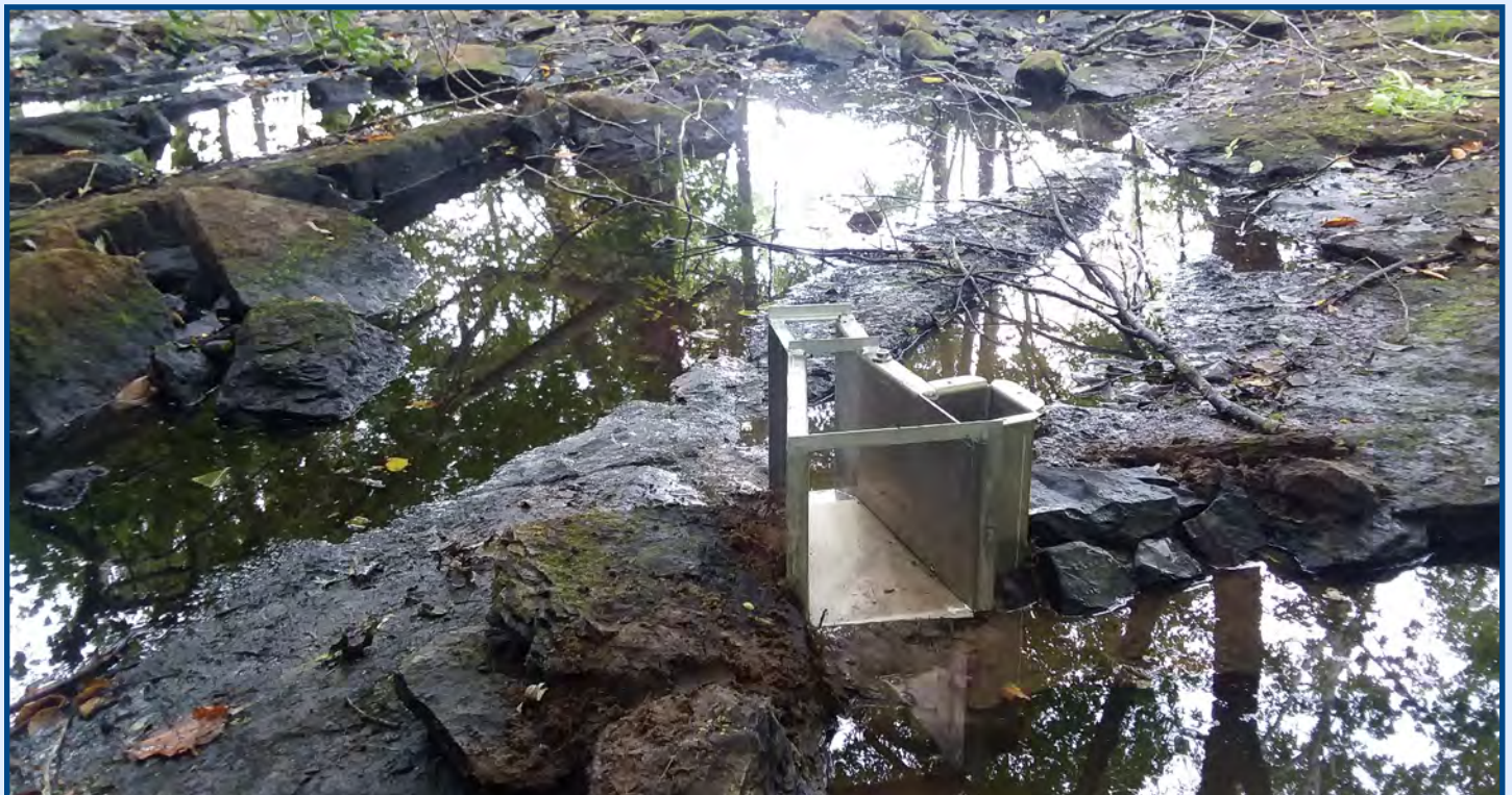
Photograph of the lowest streamflow measurement made for the period of record using a Parshall flume at Stony Brook near West Suffield, Connecticut, at U.S. Geological Survey streamgage 01184100 on September 18, 2020; photograph by the Nigel Pepin, USGS.
